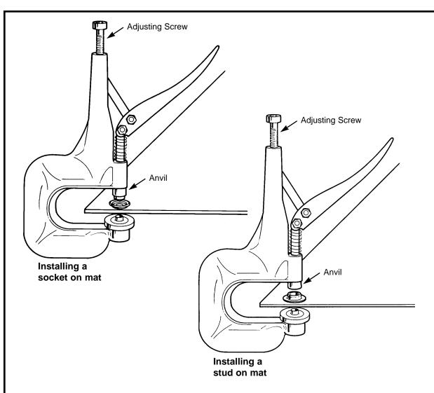
Tool includes two anvils, one for sockets, one for studs.
